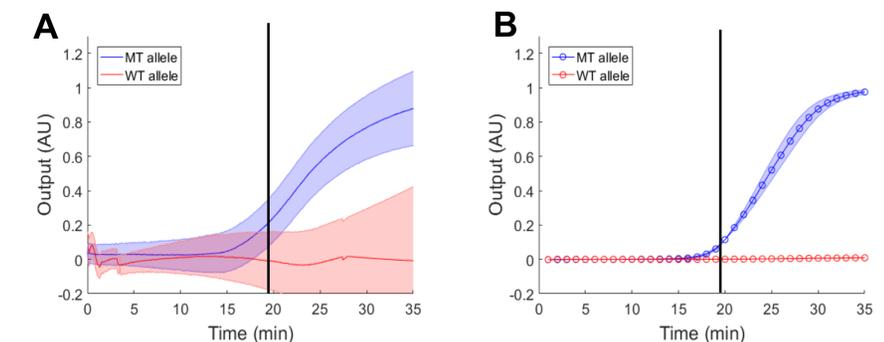
**Figure 3.** Allele-specific pH-LAMP reaction with (A) ISFET biosensing platform, showing the mean output of active pixels with standard deviation as shaded error bar, and (B) with qPCR instrument. Non-specific reaction containing synthetic DNA harbouring the WT allele (WT allele) and specific reaction containing synthetic DNA harbouring the MT allele (MT allele).
