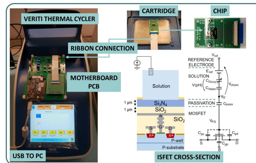
**Figure 2.** Set up of the biosensing platform and diagram of allele-specific pH-LAMP. Biosensing platform showing the microchip interfaced to a PCB with a microcontroller for data readout and the Veriti Thermal Cycler for temperature control. The reaction will only amplify the sample containing the MT allele.
